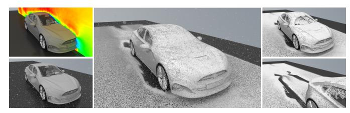
Fig. 1. Snow fall onto a car is simulated with single snow flakes modeled as single particles. The particles are coupled to a precomputed airflow field (visualized in the top left). The snow accumulates and is wiped away by moving windshield wipers. The car drives away in the end, compressing the snow below its tires.
