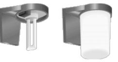
Compact fluorescent lamps for outdoor use should be in a sealed fixture with ventilation slots.
