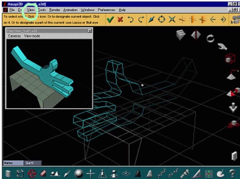
select '**Free View**'. This lets you open a free floating viewer in which you can select various display modes for interactive inspection. Click the left button and drag the mouse to examine the part. The right button moves you in/out and left/right.
