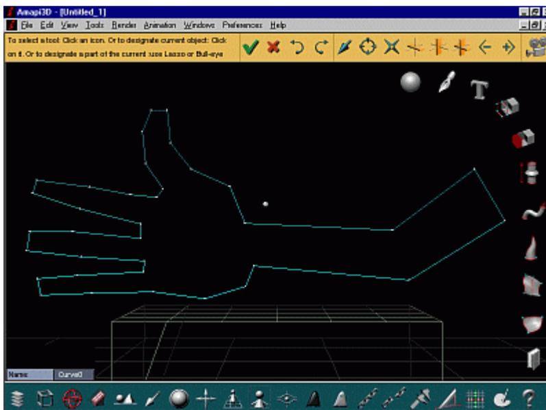
Next, use the **Arrow keys** or the **trackball** at bottom (**control panel**) to rotate the view to the side, and select the **Extrusion** tool
