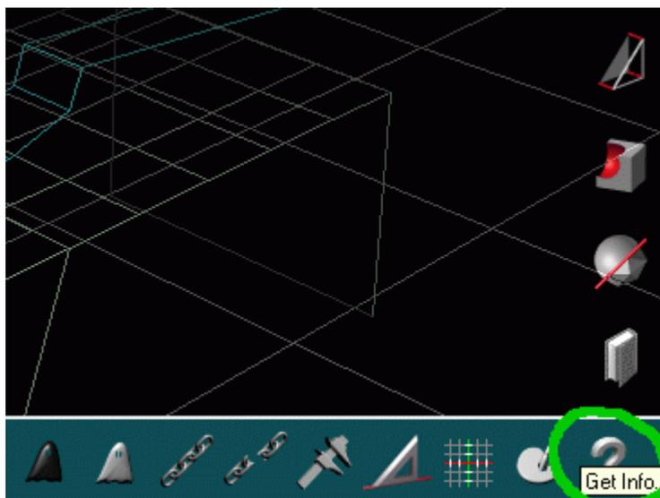
The question mark in the lower-right corner (Get Info...) does the same as if you double-click the part. It displays an info panel, which shows what type of object it is (e.g. a Volume, i.e. a closed surface in this case).
