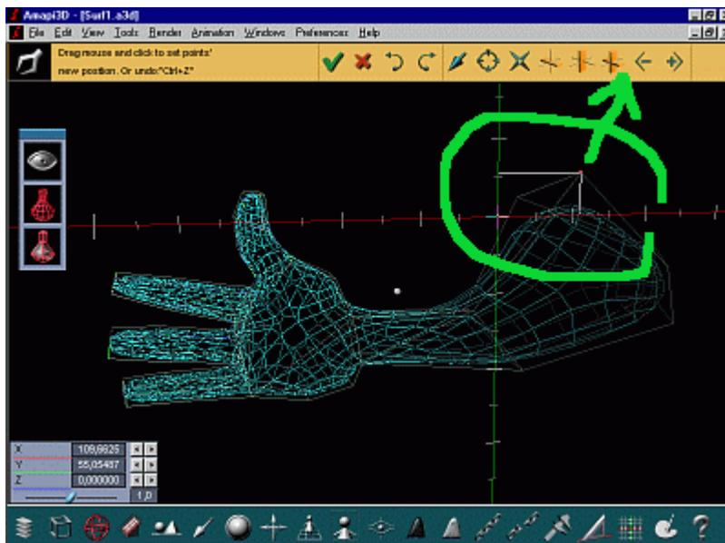
If you use the Stretch tool again, you'll be able to edit the control points of the original, coarse hull which was created by the extrusion of the profile curve. It somewhat mimics a Nurbs cage and the underlying smoothed Nurbs surface.
