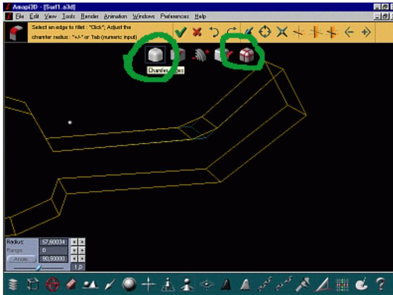
Click the right mouse button or the left-most icon in the Chamfer tool palette which pops up when you click the Chamfer tool.
