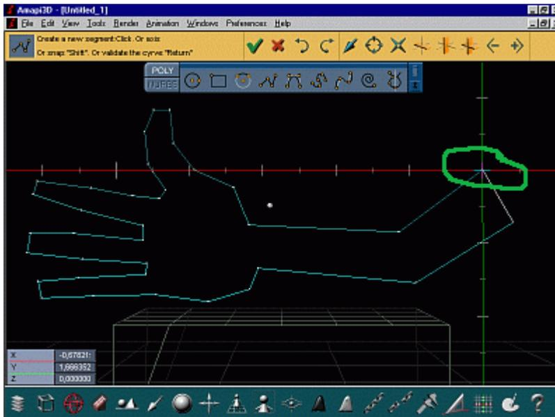
Hold the **Shift** key down while moving the cursor to the starting point in order to be sure we're **snapped** to it and close the curve by clicking on that first point.
