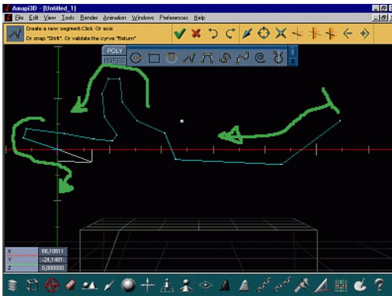
Start drawing the shape, like from the upper right corner where the arm/elbow is, and over to the wrist into the hand and thumb, then the index.
