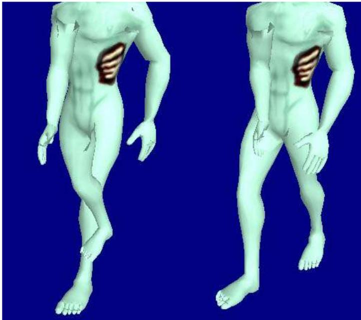
**Figure 7: Alpha Channels cause z-sorting rendering problems**
