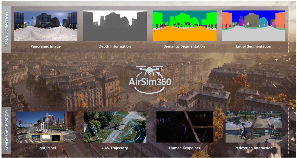
Figure 1. Overview of Airsim360. This work introduces a panoramic UAV simulation platform based on a cutting-edge rendering engine, enabling closed-loop simulation for omnidirectional aerial systems and offering an integrated toolchain for intelligent data acquisition across diverse flight scenarios.
