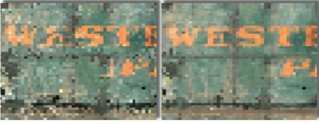
Fig. 3: One-pixel point rendering with fuzzy depth testing and threshold \alpha = 0 on the left and \alpha = 0.01 on the right. Geometric aliasing is significantly reduced due to blurring of points with similar z-values.
