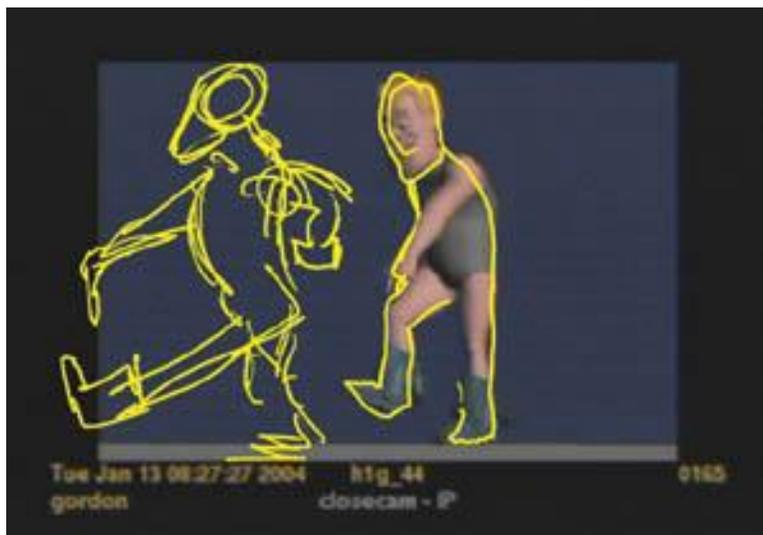
Using Pixar's Review Sketch tool, an animator can draw on an image, and then play the scene with the image moving underneath the drawing. Other features of the tool include a slider for choosing the width of the anti-aliased line, ghosting, and a raster eraser. The tool's drawings are stored on Pixar's intranet, which allows for immediate accessibility.
