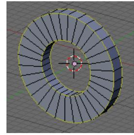
Using the Bevel Centre script and following the details given in [608 Part-4](#) add a 0.1mm chamfer. Back in vertex select mode select **All** and Set Smooth **W**, in the Modifiers tab add an Edge Split modifier with the default settings. If Black areas are present on the surface of the washer press **Ctrl-N** to recalculate the normals to the outside.
