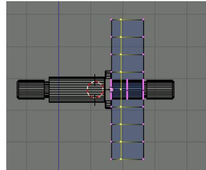
Select the flange face's, one side at a time and extrude them 10mm. The top and bottom flange will shield the components of the slide from dust produced by the router.
