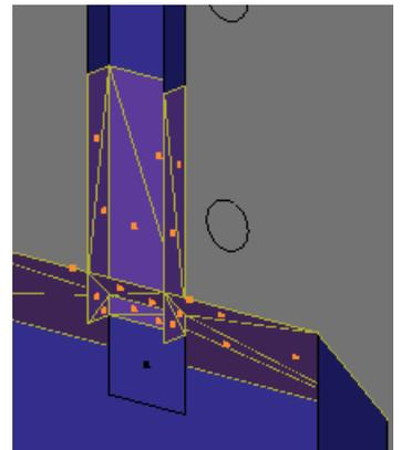
Extend the top of the slot 5mm to allow the adjuster bracket room to slide.
