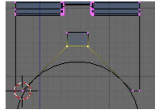
The roller profile is now ready to spin around the central axis. Select all the vertices of the profile, including those attached to the bore.
