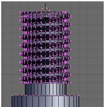
The thread is now the correct length for the axle but there is still more to do. We must join the base of the thread to the under-cut and the top of the thread to the chamfer.
