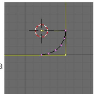
Select the vertex on the top edge above the fillet and move it **G** along the **Y**-axis **0.2mm**. Now **Extrude** this vertex **Y -0.2**, then **Grab** this and move it **Z -0.2** A 45-degree chamfer has been added to the edge.
