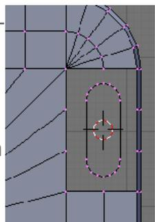
**Alt-RMB** select the vertices of the elongated hole, then **Shift-Alt-RMB** select the vertices of the flange that surround it. **Shift-F** to fill the area with faces. **Alt-F** to beautify the fill and **Alt-J** to convert to quads.
