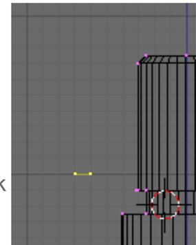
Link select both vertices of the edge and copy them **Shift-D** on the **Z-axis 1mm** (the thread pitch).
