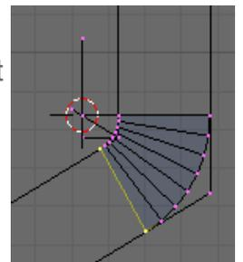
In the Mesh Tools panel set Degr:60 and Step:7 and spin the two vertices.
