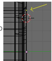
The vertex is now positioned aligned to the bearing bore and right hand edge. In side view **NumPad 3** Extrude the vertex along the **Y** axis **-17.5mm**. **RMB** select the right hand vertex and **Extrude** it along the **Z**-axis **2mm**.
