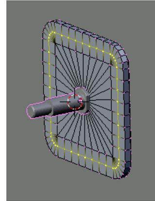
To add a chamfer to the edge of the adjuster loop cut **Ctrl-R** the outer loop of faces. With the Edge Length button activated, slide these to 0.5mm from the edge. Do this on the front and back of the flange. Now select the front outer edge loop and move it 0.5mm on the Y-axis. Do the same on the back outer edge but move this -0.5mm.
