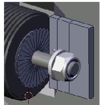
Delete some of the vertices from the outer circle and add edges back to the mounting flange. With careful choice you can get a tangential alignment.
