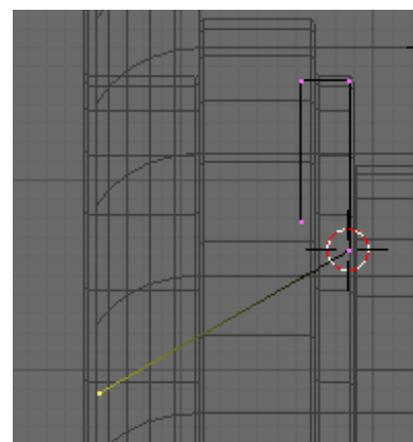
The dust shield offsets 0.85mm so extrude two reference vertices from the top corner. -0.6 then -0.25 in the Y axis
