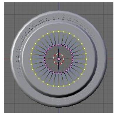
Go into edge select mode and **Shift-Alt-RMB** select the two outer and two inner edges.
