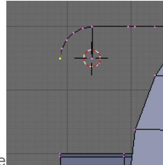
In the Mesh Tools panel set Degr:90 and Steps:5 and **Spin** the fillet radius.
