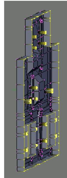
Because I haven't done any investment casting before I am not sure how thin the mould can be before it won't fill properly. Because of this I have increased the thickness behind the pockets to 4mm.
