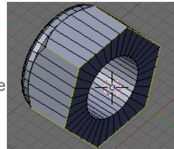
To finish add an Edge Split modifier, but because the edge angles are 30 degrees the same as the default settings for the modifier, ugly shading patterns will be created on the corners of the nut. Change the angle setting to 29 degrees to overcome this problem.
