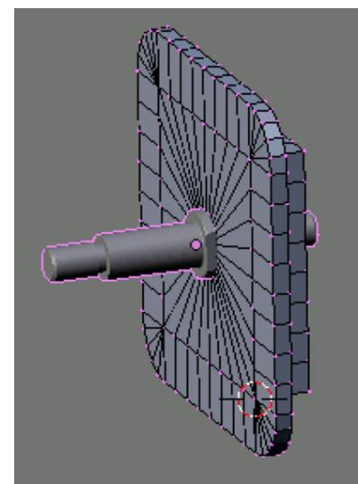
We now need the centre line of the flange to position the elongated bolt holes. It can't be loop cut because the corner faces are triangles.
