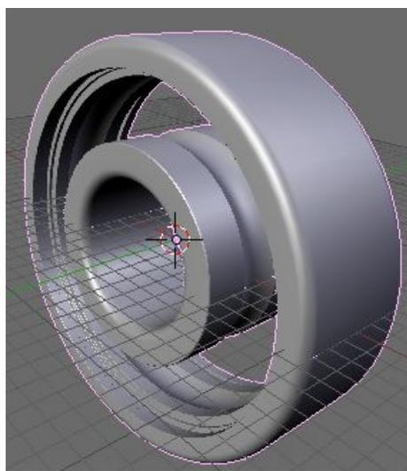
In Parts 1 and 2 we created the bearings inner and outer race, now we need to add some ball bearings. The 608 bearing has 7 balls so we will create and position one ball and then use a similar spin process to position the other six. This time though we will use "Spin Dup" to duplicate the selected vertices of the first ball around the cursor at the required step positions.
