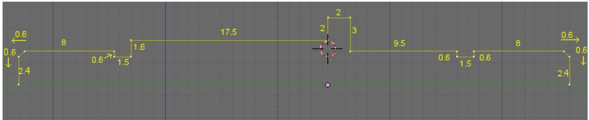
From the two edges that were positioned on the bearing bore extrude the following profile constraining the extrusions to the Y or Z-axis and dimensions indicated. The end chamfers are created by extruding 0.6mm in the Y-axis then grabbing and moving the vertex -0.6mm in the Z-axis. When complete this will form the basic profile of the axle.
