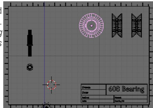
Append the V-RollerAxle from the same file and position this within the border. Copy this on the Z-axis and position it above the original. (3rd Angle projection Top view sits above Front View)
