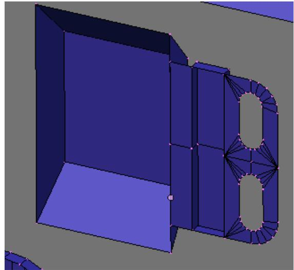
As with the V-roller adjuster, the lead screw adjusters will be secured with 4mm bolts, so the casting needs 4mm-tapped holes centrally to the slot.
