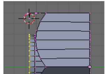
**Alt-RMB** select the inside diameters top loop of vertices and move it **G** on the **Y**-axis **0.5mm**.
