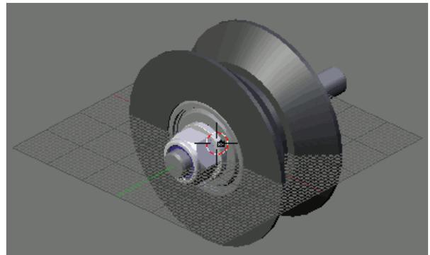
Add a cylinder to represent the shaft **SpaceBar** Add>Mesh>cylinder and in the pop-up menu set Vertices: 32, Radius: 9, Depth: 100. In its current position the shaft penetrates through the V-Roller so we need to move it down so that the shaft sits below the 'V'.
