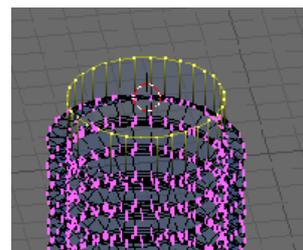
**Tab** into Object mode and in the Mesh panel click the Centre Cursor button. This will move the object centre to the centre of the top row of vertices.
