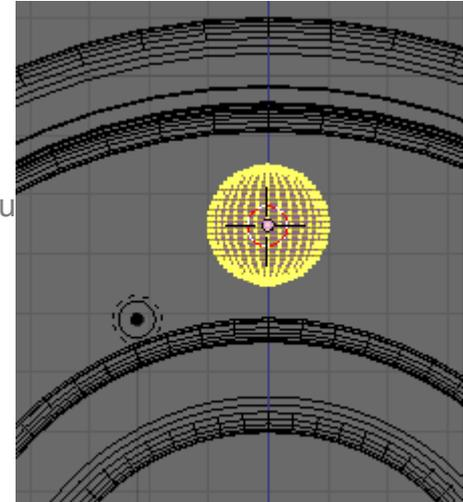
To obtain the correct scale factor, divide the required size of the ball by the inserted size of the UV sphere. As the balls are 3.95mm diameter and the UV sphere is 2mm then:  $3.95 / 2 = 1.975$ .
