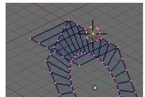
To determine the angle of the spin, with the centre vertex still selected **Shift-RMB** select the two vertices on the corner of the opposite edge and temporarily form a triangular face. With the face selected click on the **Edge Angle** button of the **Mesh Tools 1** panel. The corner angles of the triangle will be displayed in the view. The spin angle is 71.635 degrees. Press **Ctrl-Z** to remove (*undo*) the triangle
