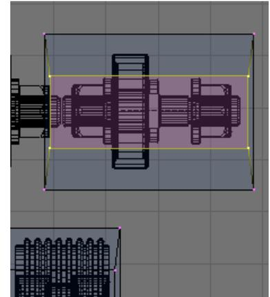
With the two recesses modelled it's easy to see where the rest of the components can be repositioned to make the casting more compact.
