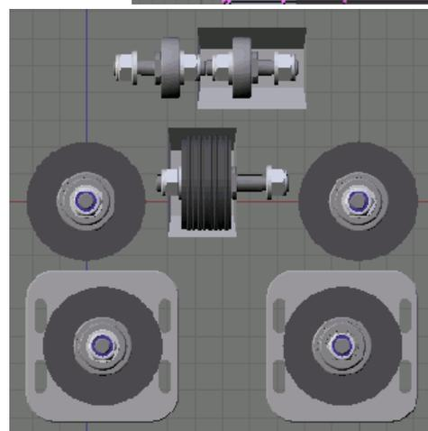
To form the pockets in the casting where the adjuster blocks sit we can copy both adjuster blocks **Shift-D** then press **Escape** to leave them in position. We can then cut and adapt the copied adjuster blocks mesh to form the adjuster locations in the casting.
