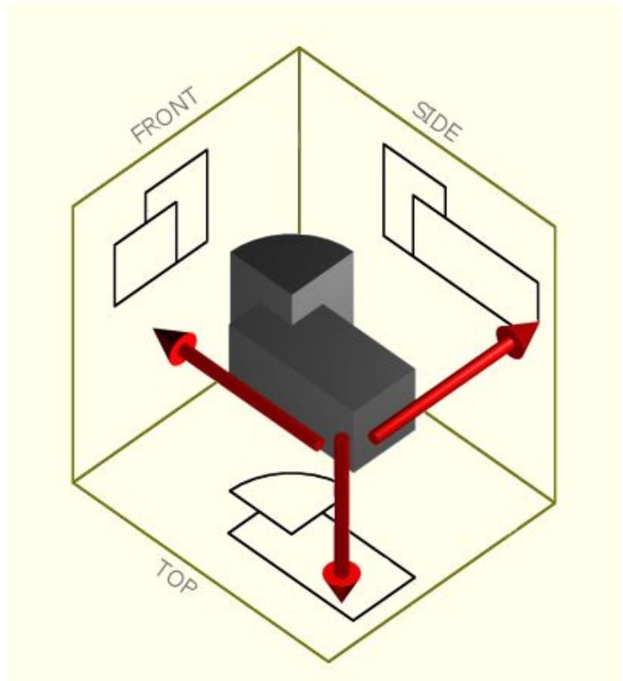
When the 1st Angle view is folded out the front view is at the back of the top view and the side view is on the opposite side of the front view. This type of layout often causes confusion with people who aren't completely familiar with orthographic layouts.
