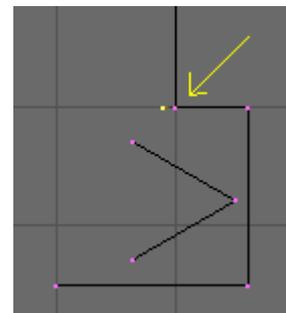
Select the vertex on the major diameter of the thread and Extrude it on the **X**-axis **-0.108mm** (1/8 H)
