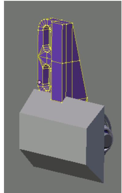
The left-hand adjuster stands out further from the casting to allow support forward of the lead screw centreline.
