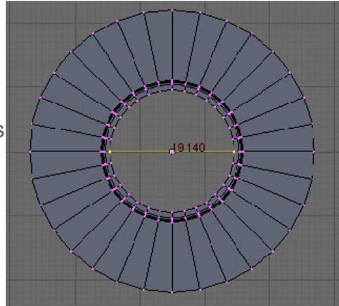
Separate this edge from the V-Roller **P**, choose "Selected" from the pop-up menu. **Tab** into Object Mode and select the new edge, which will be used to form the dimension line. Go into Local view **NumPad /** for dimension line, then **Tab** into Edit Mode (Note I have removed the material to make the images clearer for this tutorial).
