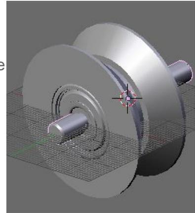
The nut should also impart a small amount of pre-load onto the bearing to remove any side play. In true skateboard fashion I am going to use a 6mm nyloc-locking nut and washer.
