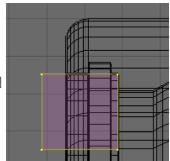
Grab **G** the end vertex and move it along the **Y**-axis **1.75mm** so the top edge measures **0.25mm**, the thickness of the dust shield.
