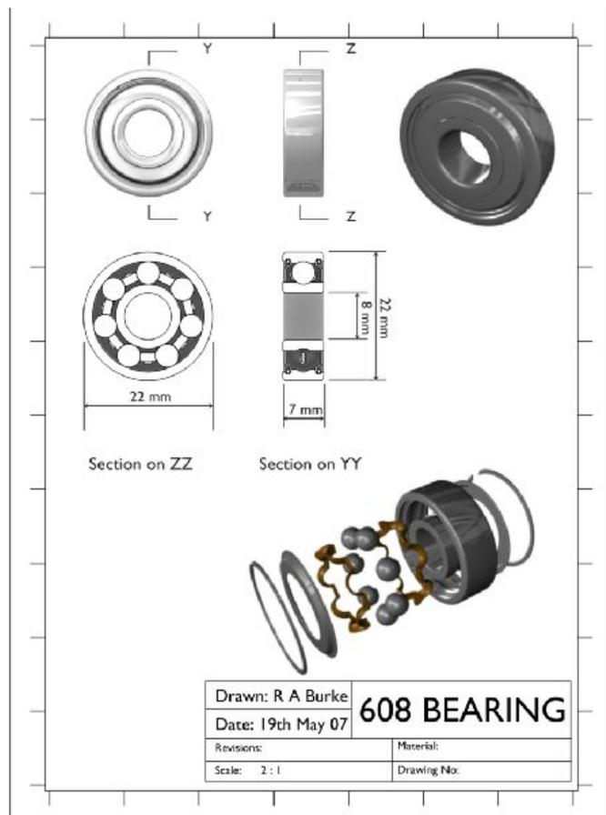
The final result gives a good layout drawing, easily capable of communicating the essential elements of a product design. With sufficient planning and forethought any component could be created, rendered and dimensioned in Blender.
