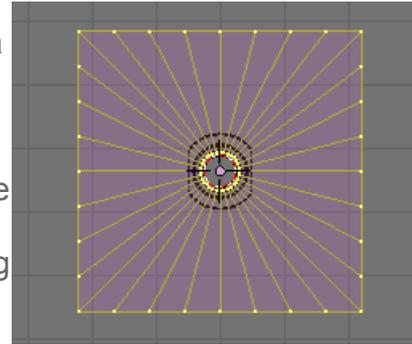
In order for the adjuster block to be able to be positioned in the casting it needs some side flanges that will also incorporate the elongated bolt holes. In side view **NumPad 3** cut a loop of vertices **K** "Midpoint". **G**rab the new loop of vertices and move them on the **Y**-axis **-2**mm, this will give us a 3mm face to form the flange from.
