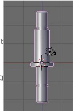
Copy these vertices **Shift-D** then **Esc** to leave them in place. Separate the copied vertices from the Object **P**. Its easier to work on the separated profile rather than the complete axle.
