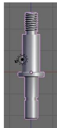
In front view **Box** select the thread vertices, then loop select **Shift-Alt-RMB** the inner loop of vertices on the undercut next to the main body of the axle.
