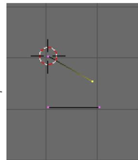
Then select the vertex on the other end of the edge and with the Pivot set to 3D Cursor **Rotate** it **30** degrees.
