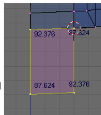
To form the clasp we need to spin the bottom face 92.376 degrees. Select only the bottom two vertices and delete them **X** as they were there just to obtain the required spin angle.
