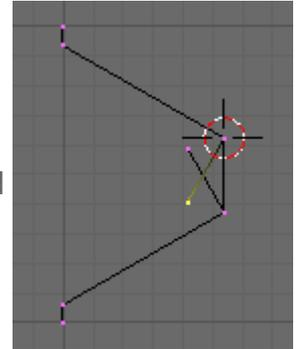
Again **Shift-RMB** Select both vertices of the minor diameter and copy them **Shift-D**, then **Esc** to leave them in place. This time **Rotate** the edge **30** degrees.
