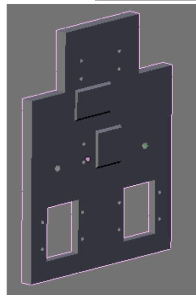
Select the loop of faces from around the outer edge of the inner face. These will be extruded to provide a mounting point for the Y-axis and also offer some protection to the components of the X-axis.
