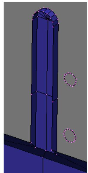
The left-hand adjuster slot just needs to be extended 5mm top and bottom.
