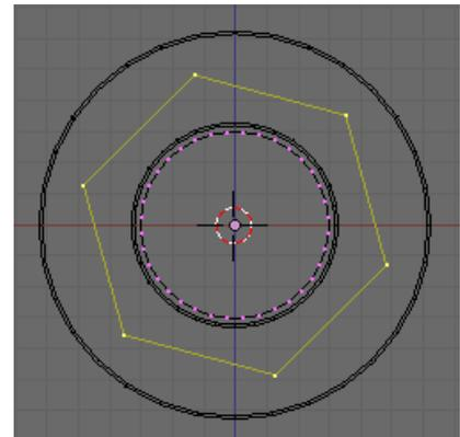
Some extra detail on the external profile will be required to form the curves on the top edge of the nut so it would simplify the modelling to keep the same number of vertices on the outer and inner diameter.
