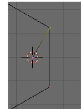
Select the vertex at the top of the major diameter and in the Mesh Tools panel set Degr:120 and Steps:4 Press Spin and the profile for one pitch of the thread will be created.
