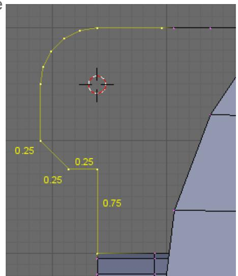
Form the chamfer by **Extruding** the vertex **Y -0.25** then **Grabbing** this vertex and moving it **Z 0.25**
