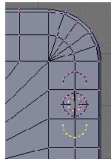
Copy the vertices from the circles centreline and above and move the copy 4mm on the Z-axis. Then copy the vertices of the circle from the centreline and below moving them -4mm on the Z-axis.
