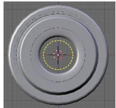
**Extrude (Only Edges)** this vertex ring then press **Esc** to leave it in place. We will scale the extruded vertices to form the outside diameter.
