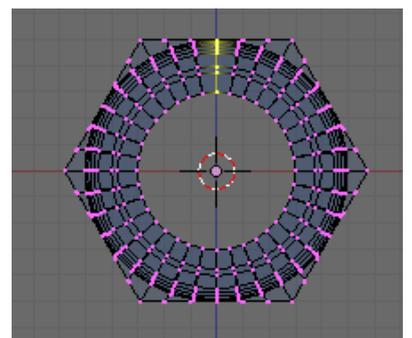
In the Mesh Tools panel set Degr:360 and Steps:36 and **Spin** the top profile.
