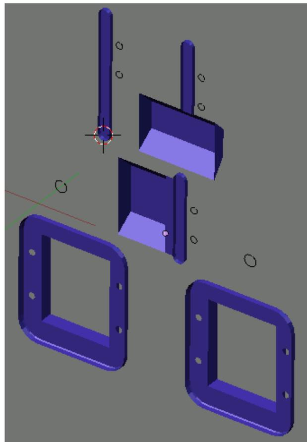
With the location of the bolt holes, Key way slots, adjuster housings and recesses now positioned all that remains is to build the face of the casting between the edges already modelled.
