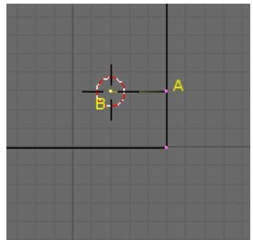
In the Mesh Tools panel set Degr:90 and Steps:5, then press Spin. The corner fillet will be formed.
