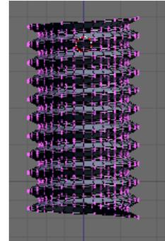
Go into top view **NumPad 7**. De-select **All** then **Link** select the centre and chamfer vertices. Delete these **X**.
