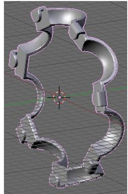
The dust shield will be formed in the same way as we made the bearing inner and outer race. We will create a section through the dust shield and spin this around the bearing centre to form the 3D component.
