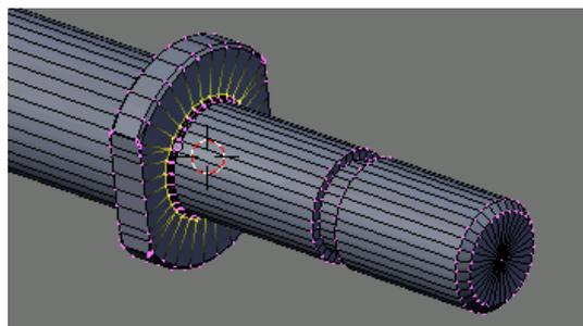
Select the axle location circles, the pockets behind the roller-nut and bearing and the adjuster recesses and combine them into one mesh, **Ctrl-J**.
