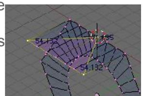
In top view NumPad 7 select the bottom right hand vertex indicated and in the Mesh Tools panel set Degr: 71.635 and Steps:6.
