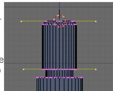
Go into edge select mode and paint a selection **B B** across the straight section of the thread.
