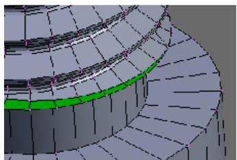
To correct this we need to manually merge the vertices of the original axle flange onto the corresponding vertex of the thread.
