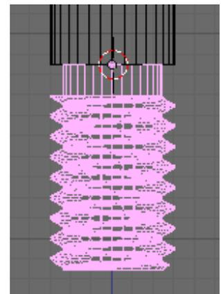
With the thread still selected **Shift-RMB** select the axle and join the two objects into one **Ctrl-J**.
