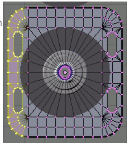
In scaling the adjuster on the Z-axis we have also just scaled the slotted bolt holes. These need to be returned to their original size. We can do this by scaling the vertices of the slots by the inverse of the original scale ( $1 / 1.2222 = 0.81818$ ).
