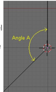
To work out the centre point of the fillet we simply construct a right angle triangle with half angle A and the radius. The hypotenuse is the distance to the centre point at an angle of half A
