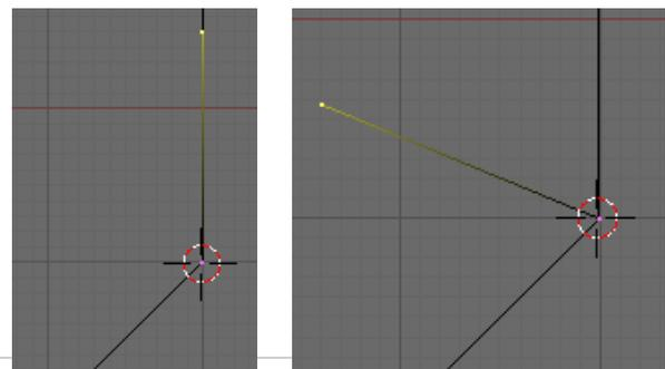
From the intersect extrude a vertex perpendicular to the edge on the known axis and the length of the fillet radius.
