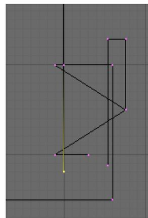
Select the three vertices of the V and cut **Knife (Exact)**, snapping the cut **Ctrl-LMB** to the vertices of the major diameter.
