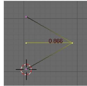
Delete **X** the vertex on the left-hand side of the central edge. Select the three vertices of the thread profile and move **G** them towards the undercut at the bottom of the thread.
