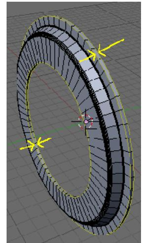
A Dust shield will also be required on the other side of the bearing. Rather than repeating the modelling process we will duplicate this dust shield and Mirror it across the bearing centre.
