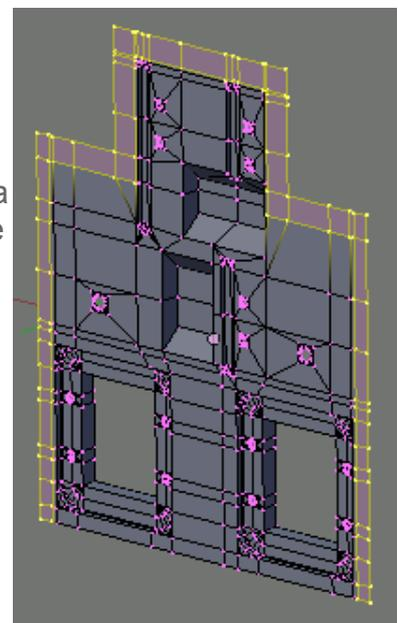
Extrude the holes and the outer edge back to give the casting thickness.
