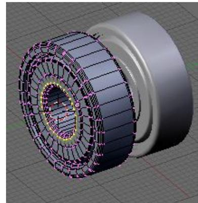
Press the **Spacebar** to open the Toolbox and select Add>Mesh>Circle. From the pop-up menu leave vertices at 32, but change Radius to 3.2 then press OK to accept. This will form the 6.4mm inside diameter of the washer.
