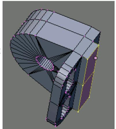
The support bearing adjusters are modelled in a similar way to the Roller-nut adjuster bracket. I have slimmed down the bracket to 6mm and moved the mounting flange above the bearing.
