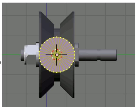
**Tab** into Object Mode then **G**rab the shaft and move it on the **Z**-axis until it sits just below the V-Roller. Zoom in fully and repeat this if necessary to get the closest possible alignment. You can also zoom into a selection box by pressing **Shift-B** and dragging a selection box over the zoom area you require.
