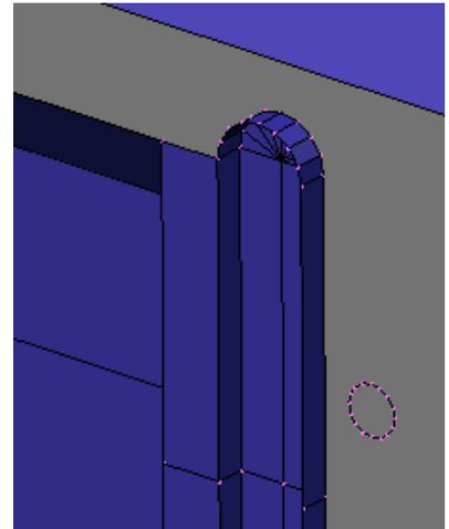
The slot on the top right adjuster poses a different problem, as it has to penetrate the face of the bearing recess.
