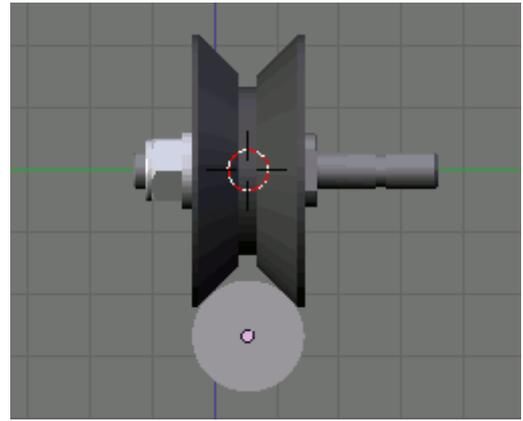
In front view **NumPad 1**, **Tab** into Edit mode and **B**ox select the right-hand vertices. Move these vertices **G** along the **X**-axis **300mm**. This will make the shaft 400mm long. **Tab** back into Object Mode.
