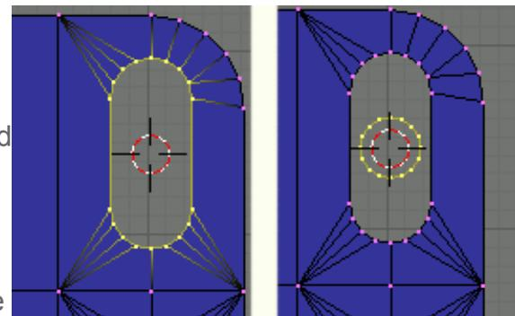
Delete the unnecessary vertices, leaving the key way slot and tapped hole circles.
