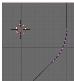
Getting back to the dust shield we will use the reference geometry method to position the fillets with a small radius of 0.1mm and a large radius of 0.35mm. The angle between the edges is 120 degrees.
