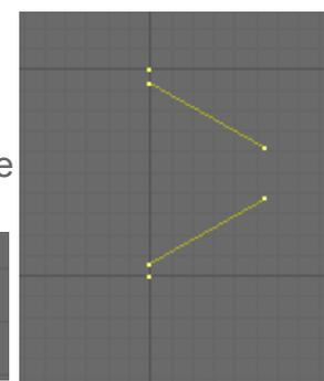
Add Edges **F** to the vertices of the major and minor diameter. Threads usually have a radius at the root of the thread so we will add a fillet.
