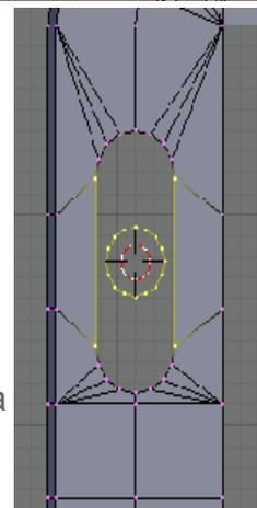
Delete the vertices of the slot then rebuild the faces around the hole.
