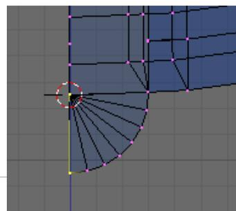
Re-select the newly spun face and Extrude **E** (Region from sub menu) and **0.3** for the distance. When you select region a new face will be extruded constrained to an axis perpendicular to the original face.
