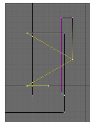
Delete the reference vertices, but ensure the top chamfered edge of the thread is not deleted, as this will be used to locate the cursor when we spin the thread.
