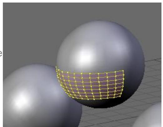
Currently the vertices of the cage are sitting on the surface of the ball which would stop the bearing from turning, so we need to add some clearance. To achieve this we will scale the cage from the centre of the top ball bearing.
