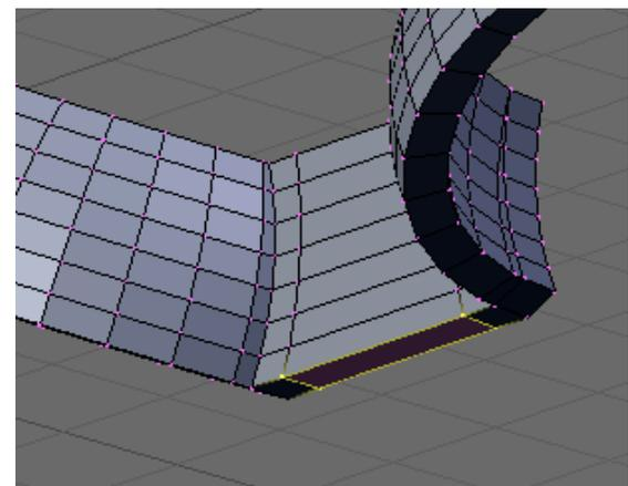
Switch to top view and go into wire view mode **Z**. you will see the selected edges are not square because they were cut from geometry originally created from the ball bearing's UVsphere, so we need to square up the edges.
