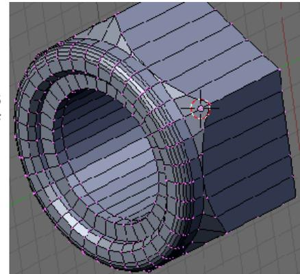
In Edge Select mode **Alt-RMB** select the bottom edge of the nut, then **Shift-RMB** select the 6 corner edges. We will add a 0.1mm chamfer to these using the Bevel Centre script described in [608 Part-4](#).
