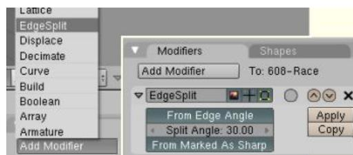
You will notice though that there is not a sharp edge between the bearing groove and the inner edges of the race because the angle is less than 30 degrees. This can be corrected by marking these edges for the Edge Split modifier to recognise as sharp.
