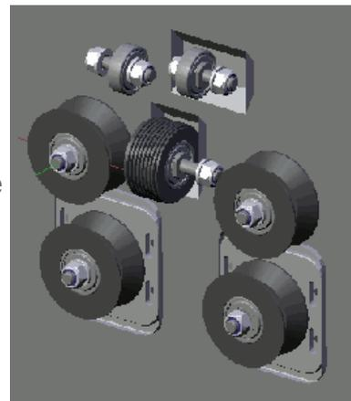
To position the fixed axle holes, **RMB** select a fixed axle and go into Local View **NumPad /**. Select **Shift-Alt-RMB** the loop of vertices at the back of the fillet and snap the cursor to the centre of them, **Shift-S** Cursor>Selection. This gives us the location point for the adjuster. Go into Object Mode and in front view Insert a mesh circle, **SpaceBar** Add>Mesh>Circle, in the pop-up menu set Vertices: 32 and Radius: 3. Repeat this for the other axle.
