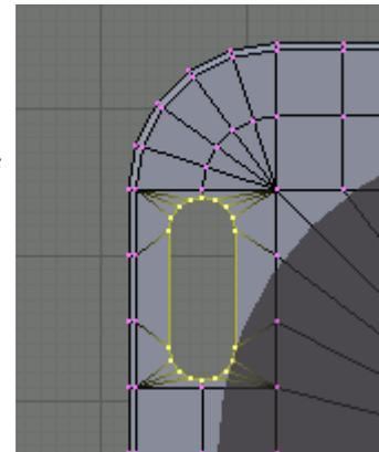
Finally scale the centre hole on the X and Z-axis by the same amount to return the hole to the correct diameter. (**S**cale **Shift-Y 0.81818**)
