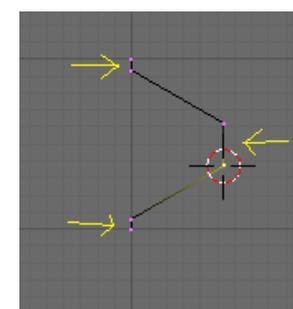
**Shift-RMB** Select both vertices of the minor diameter and copy them **Shift-D**, then **Esc** to leave them in place. With the Pivot in 3D Cursor **Rotate** the edge **-30** degrees.
