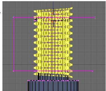
**Tab** into Edit Mode and De-select **All** then **Link** select the thread. With the Knife tool, cut two rows of vertices across the thread, **Knife (Exact)** and snapped **Ctrl-LMB** to the reference edges.
