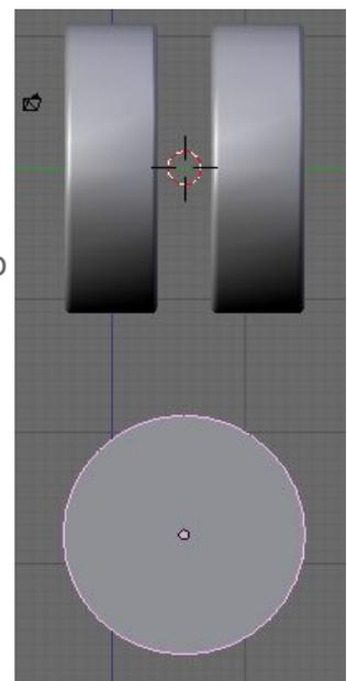
We will now use the outer profile of the bearings to form the bore of the V-roller. **Shift-RMB** select both bearings and copy them **Shift-D** then press **Esc** to leave the copy over the top of the original bearings. With the two new bearings still selected join them into one object **Ctrl-J**. In the Link and materials panel rename the object OB:V-Roller. Press **NumPad /** to go into local view for the V-Roller and **Tab** into Edit Mode.
