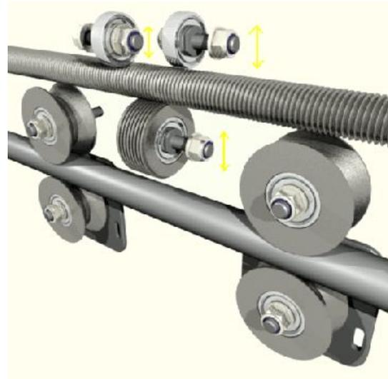
The roller-nut and bearings will also need to be adjustable, so the brackets that hold them back to the main casting will also need to allow some movement in the Z-axis.
