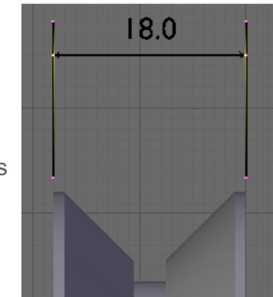
To add the dimension select the two vertices on the inner edge of the extension lines. Open Blender Caliper, adjust the measurement settings for the dimension line and press measure. (You may need to play with the settings to get a suitable font size and dimension line scale).
