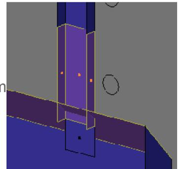
The Geom Tool will cut a new series of edges around the intersection. It will also triangulate all the selected faces.
