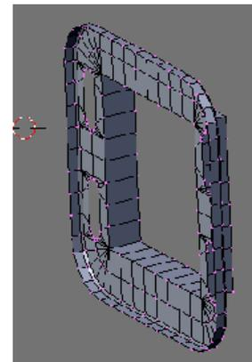
Select the vertices of the top flange and **G**rab them moving them on the **Z**-axis **4.5mm**. Move the bottom flange **-4.5mm**. This will give us the room for the adjuster block to move up and down.
