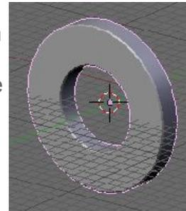
The washer is complete but before going into Object Mode we need to set the cursor ready to add the final component. **Alt-RMB** select one loop of vertices on the left hand side of the washer and snap the cursor to the centre of these. **Shift-S** Cursor>Selection.
