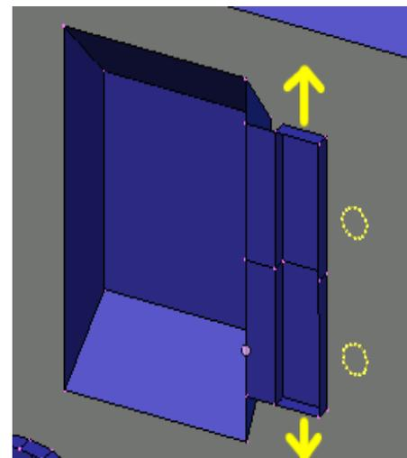
I have also cut the slot lengthways with a mid point cut. This has enabled me to spin a radius at the top of the slot, which on the casting will be cut using a 6mm slot drill, giving the radius on the ends.
