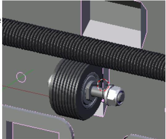
Tab into Edit Mode for the casting and snap the cursor to the front face. I have selected the two vertices of the recess, so the cursor is on the edge of the recess and aligned with the mounting face of the axle.
