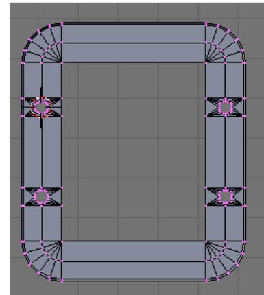
Once one adjuster recess is complete, copy it and move it 88mm on the X-axis so it sits behind the other adjuster.
