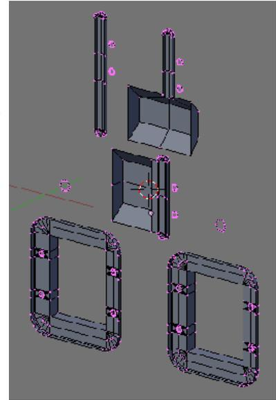
Section off areas of the casting by extruding edges horizontally or vertically. Snap the cursor to existing vertices and in cursor select, Scale the other required vertices along their axis to 0 to align them.
