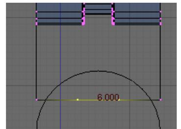
In order to cut the angles on the roller we first need to cut a central groove. On my lathe I will do this with a 3mm parting tool. To add the groove select the two central vertices. Change the Pivot to "Median point" and scale them by a factor of 0.5
