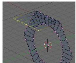
To form the radius on the top of the side face we need to spin a vertex from the faces bottom centre vertex. Select the vertex indicated and snap the cursor to it.
