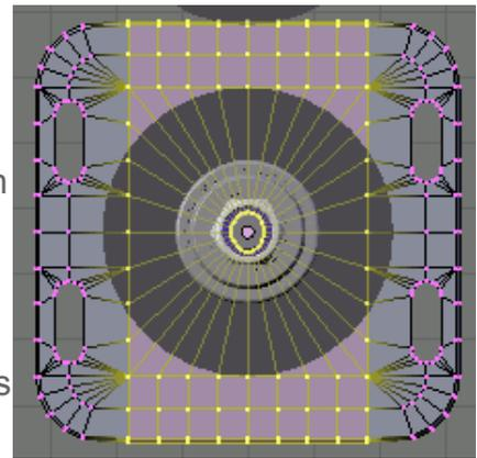
Now box select the vertices of the right hand flange and move **G** these on the **X**-axis **-4mm** ( $1/2$  the 8mm difference).
