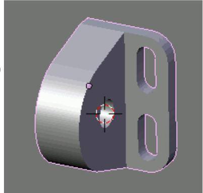
To achieve this I have purposefully created vertices that will allow the incorporation of a key, which will be located in a slot machined into the face of the casting.
