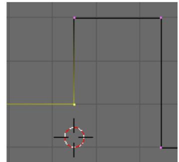
Select the inner corner vertex indicated and **E**xtrude this in the **Z**-axis **0.3mm** to point A (*vertex to spin*), then extrude this vertex to point B (*fillet centre*).
