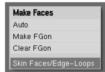
Pressing the Skin option will automatically build faces between the two vertex loops. It works the same as the Loft function in many 3D CAD packages.
