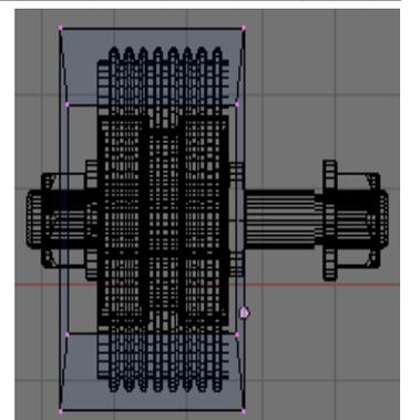
In top view move the back side vertices in 1mm to add a withdrawal taper.
