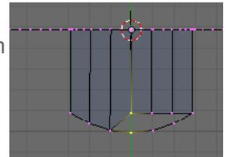
Merge the rest of the vertices on the top edge of the nut face to the ark using this method.
