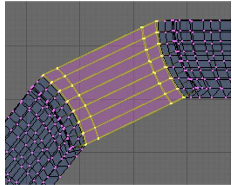
Ensure the cursor is still on the bearing centre axis and Spin Dup the selected vertices. Degr: 360, Step:7.
