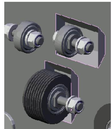
There's plenty of room to allow me to move the V-roller centres from 150mm to 110mm. It's also apparent the Adjuster blocks are larger than they need to be so I will reduce their size.
