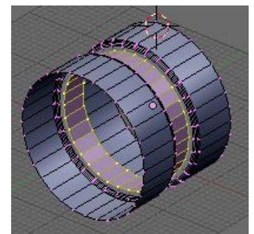
The bore of the V-Roller could be called finished at this stage, but its not really good engineering practice to have the inner fillet radius of a bore the same size as the object that is going to fit into it.
