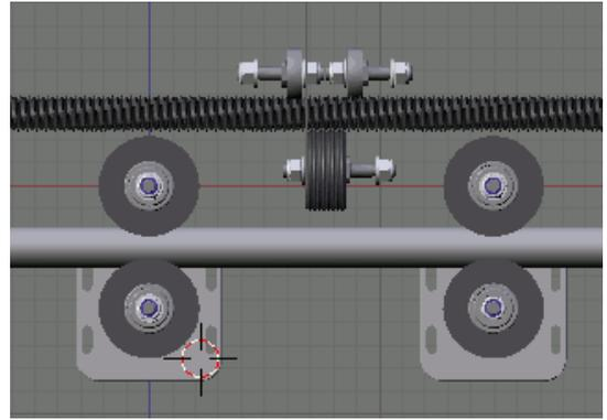
In side view its clear that some of the components will penetrate the front mounting face of the casting. It will be necessary to provide a recess behind the roller nut and top right hand bearing.
