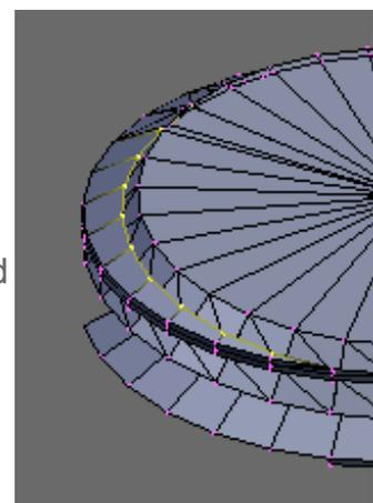
Only delete **X** a few vertices at a time, if necessary **Ctrl-Z** will undo the change. In places you may need to merge vertices **Alt-M** and other places you will need to add new faces **F**. Its also worth noting on one side of the axle the thread intersects the chamfer in two places.
