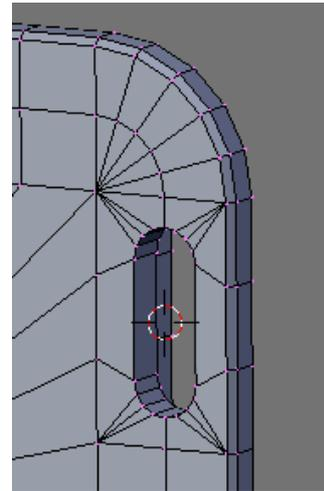
Select the vertices central to where the other three slots are required and delete them. Copy the slot faces and surrounding faces. and use Blenders snap tools to snap the copy to the other locations.
