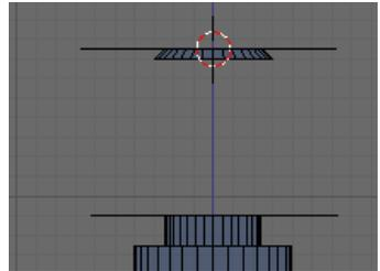
**Tab** into Object Mode and in the Outliner bring the thread back into view. **RMB** select the thread then **Shift-RMB** select the axle. Press **Ctrl-J** to join them into one mesh.
