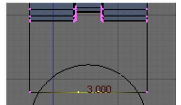
To give a small flat at the edge of the V-Roller **Extrude** the bottom left corner vertex in the **-Z** direction then **Extrude** this vertex in the **Y**-axis **1mm**, then **Extrude** this vertically crossing the bottom edge. This will be used to cut a new vertex 1mm from the corner of the bottom edge.
