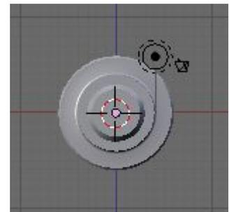
The screw tool spins a profile around the Z-axis so the profile needs to be created and the screw operation performed in front view. The Axle needs to be rotated so it is vertical in the front view. **Rotate X -90**.
