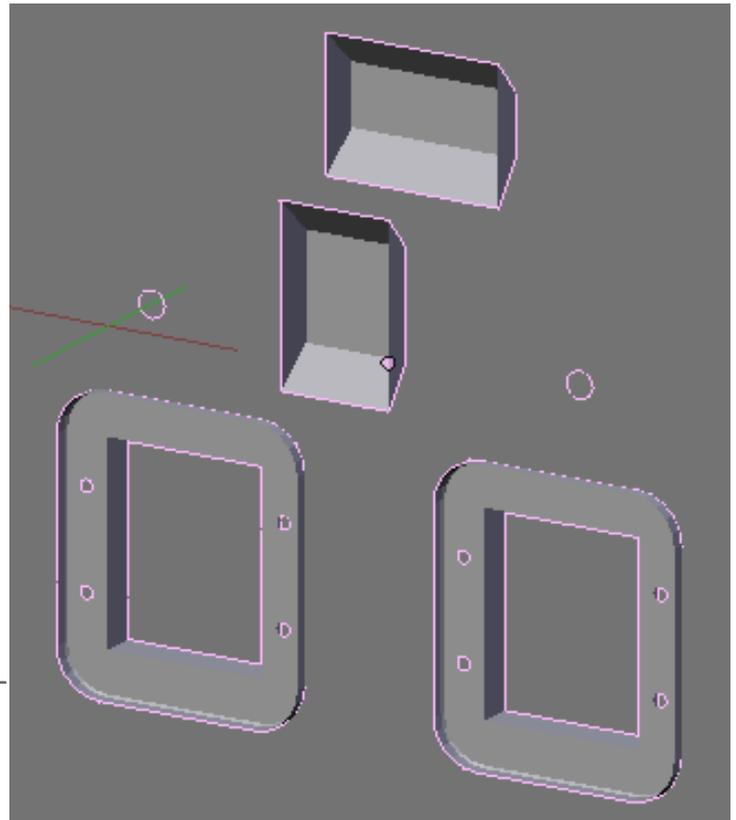
To finish off all the mounting locations on the casting, we need three more components, the mounting brackets for the Roller-nut and support bearings. Because the design of the brackets relies on the position of the casting face from the axle centres and also any pockets in the casting, it has not been possible to design the brackets until now.
