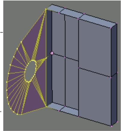
As detailed in Part-1 for the V-roller adjuster brackets add two elongated holes to the flange and also a fillet to the outer corners.
