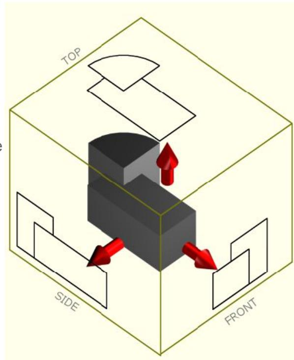
In 3rd angle projection the views are positioned on the same side of the view next to them, so the top view is on top of the front view and the side view is on the side of the front view that it represents. This is a much easier layout to understand and my preferred choice.
