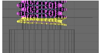
De-select **All** then **Box** select the vertices below the bottom reference edge. Zoom in **MW** to make sure all the vertices below the edge are selected (*not the vertices on the edge*) Delete these vertices **X**.
