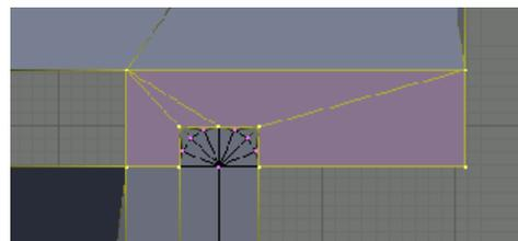
By constraining regions vertically and horizontally you can construct an organised mesh. The advantage of doing this are that if alterations are required to the model selection of aligned rectangles will be much easier than selecting areas of a mesh made up of disorganised triangles.
