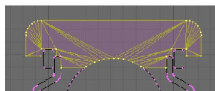
Link select **L** each closed area of the slice and fill the area **Shift-F** with faces.
