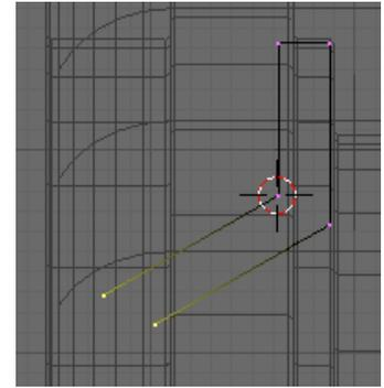
Before we extrude them we need to set the cursor on the top of the inner bearing race. **Tab** into Object mode and select 608-Race. **Tab** back into Edit Mode for this object. Select a vertex from the top of the inner race **RMB** and snap the cursor to this, **Shift-S** Cursor->Selection.
