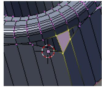
Select 4 vertices (*3 on the corners of the openings*) corresponding to where a face should be and press **F** to insert a face. Continue around the perimeter of the nut until all faces are filled.
