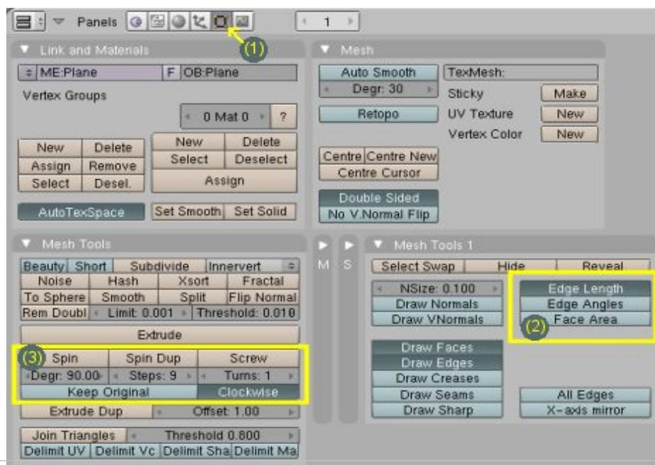
The bearing has a 0.6mm fillet on the edge of the inner and outer race. As Blender is not primarily a CAD program it doesn't yet have a dedicated fillet tool. However it is both quick and simple to add a fillet using the Spin function (3) in the Mesh Tools Panel
