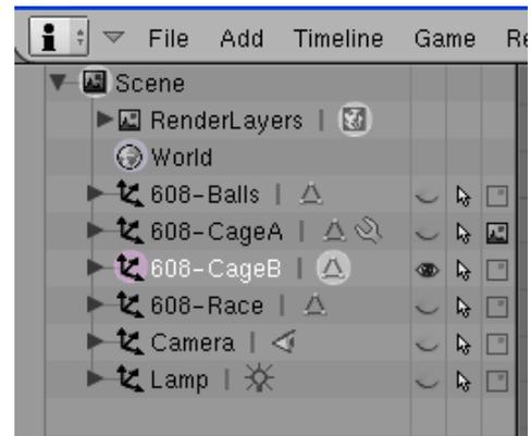
When we originally mirrored the cage from 608-CageA, we effectively applied a scale factor of -1 in the Y axis. Press **N** to open the Transform Properties window, You will see ScaleX:-1.000. To clear this back to ScaleX:1.000 we need to apply the scale to the object. To do this press **Ctrl-A** and accept "Apply Scale and Rotation". If you had simply changed the number in the Transform Properties window to 1 the cage would have flipped back to the other side of the bearing
