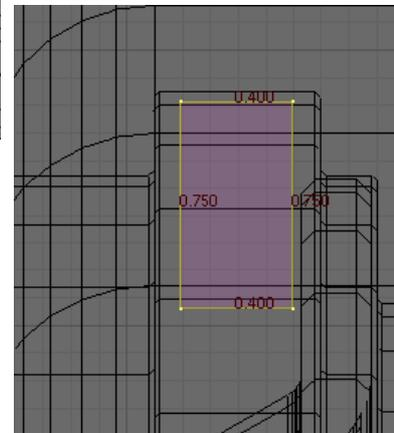
Go into front view **NumPad-1** and spin the vertices around the bearing centre. In the Mesh Tools panel Set Degr:360 Step:64.
