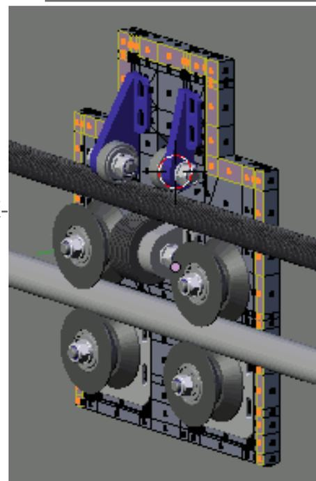
This completes the casting for the X-axis of my CNC router. All that remains is for me to make a wax pattern, which will be fabricated, from templates printed at a scale of 1 to 1 from the Blender model.
