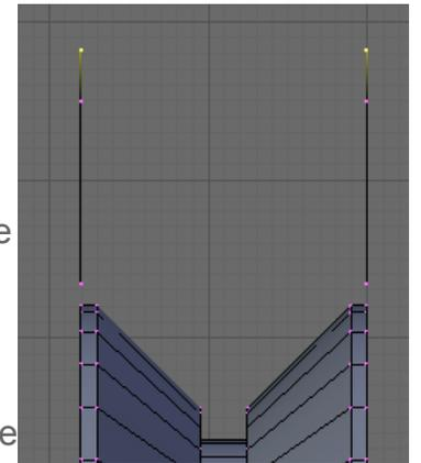
To thicken each edge so it will show on the render, select the three vertices of one edge and extrude it away from the other edge 0.2mm. Do the same with the other edge.
