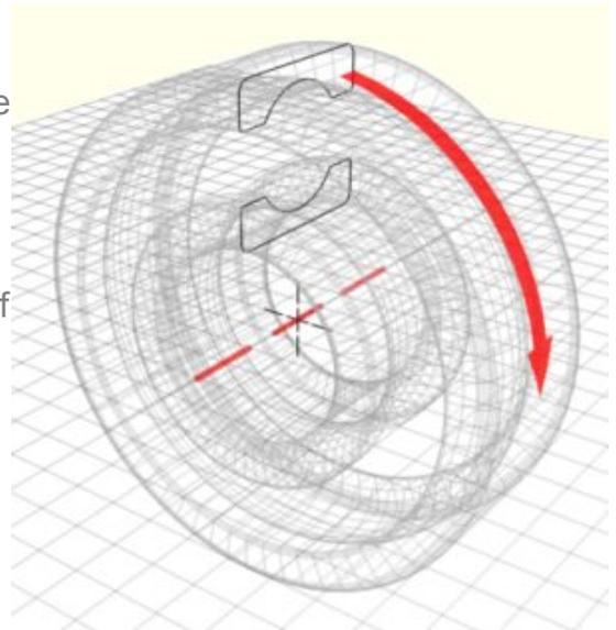
The method to create the shell of the bearing will be to draw a cross section of the inner and outer race relative to the centre of the bearing and then spin this through 360 degrees.
