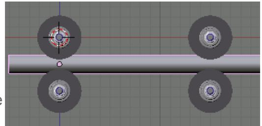
Its not feasible in a home workshop to make components to micron accuracy so some form of adjustment will be necessary to position the V-Rollers tight to the shaft. I am going to fix the top two rollers into the main casting, but allow the bottom rollers to be adjusted on the Z-axis. For this I will use a simple rebated block with elongated bolt holes. This can simply be located within a rebate in the main casting.
