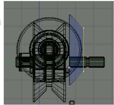
I have repeated the process for the top Right-hand bearing. This time making a little extra room for the axle and nut which also penetrate the front plane of the casting.
