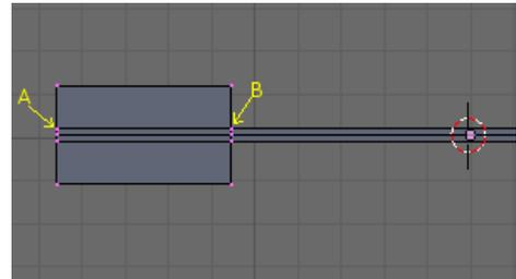
Select the six new vertices that have been cut and **Scale** them along the horizontal edges **X** until they are around 4mm from the ends of the dimension line. Select the two vertices A & B and **Extrude** them in the Z axis 1mm Repeat this on the other three edges. You should end up with a dimension line that has a box on either end.
