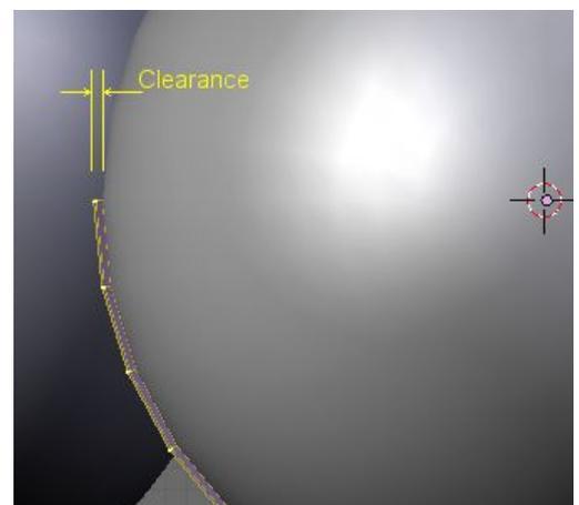
**Tab** back into Object Mode and select the Cage and **Tab** back into Edit mode. Make sure the Pivot Point is set to 3D Cursor and scale **S** the cage 1.02 This will give you a clearance of 0.0395 between the ball and the cage.  $((\text{Diameter} * 1.02) - \text{Diameter}) / 2$
