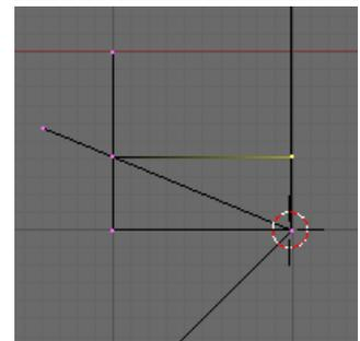
Set the cursor on the centre point and spin the vertex on the end of the radius edge through an angle of
