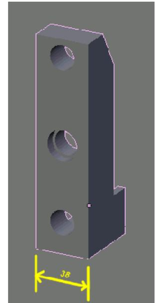
As part of the casting's inner face I have incorporated a loop of faces around the outer edge, these will become a flange to help stiffen the casting and also give the mounting location for the Y-axis support bracket.
