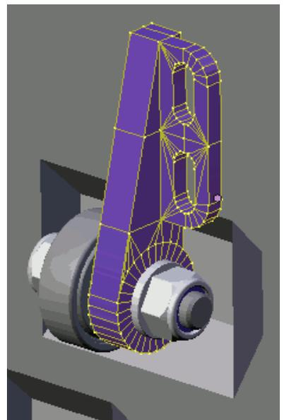
The view from the back shows the 6mm key, which penetrates the face of the casting.
