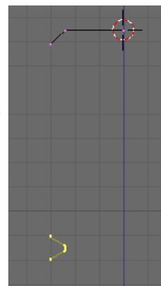
Select **All** and Remove Doubles **W**. Select the vertex on the thread centreline (right hand vertex on the top chamfer profile) and snap the cursor to it.
