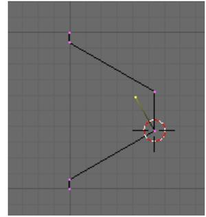
Select the vertex at the top of the minor diameter and snap the cursor to it **Shift-S** Cursor>Selection.
