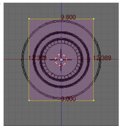
Select **All** and **Scale** the Plane on the **Z**-axis till it is larger than the flange.
